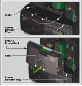
FIGURE 8. SMART POWERPACK PLACEMENT
